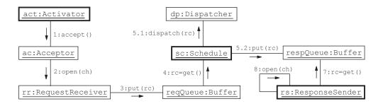
Figure 5: Representation of the main components of Arcademis.
