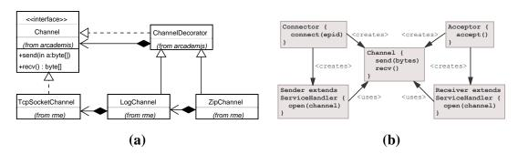
Figure 2: (a) Composition of decorators. (b) The acceptor-connector components.
