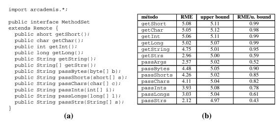
Figure 8: (a) Interface for performance tests. (b) Performance results: requests/s.
