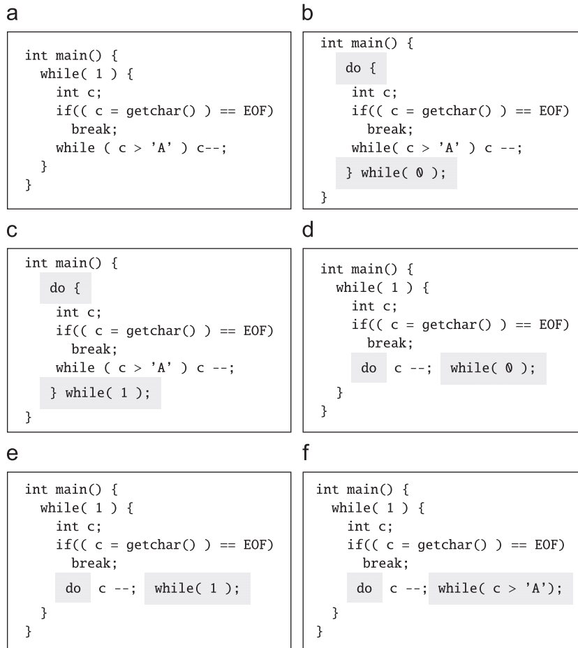
Fig. 19. (a) Original program. (b)–(e) Mutants generated by operator in Fig. 18. The mutated parts of the code are highlighted.
