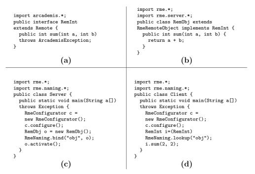
Figure 8: (a)Remote Interface. (b)Remote Object. (c)Server. (d)Client.
