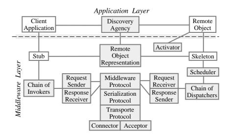
Figure 2: Representation of the main components of Arcademis.
