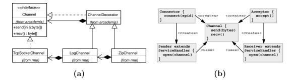
Figure 3: (a) Composition of decorators. (b) The acceptor-connector components.
