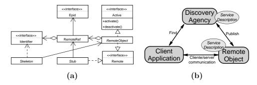
Figure 5: (a) Components for remote object representation. (b) Service-oriented architecture.
