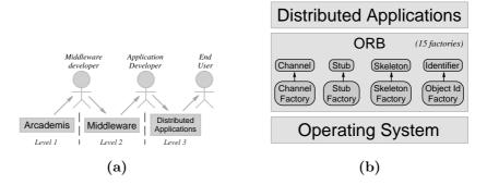
Figure 1: (a) The programming level views. (b) The ORB organization.
