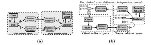
Figure 4: (a) Request-response. (b) Example of server configuration.
